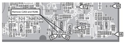
Figure 2 T800 Transmitter Audio Processor - Top Side
