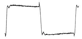
Figure 5 100Hz VCO Control Line Waveform
