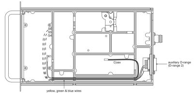
Figure 3 Cable Routing
